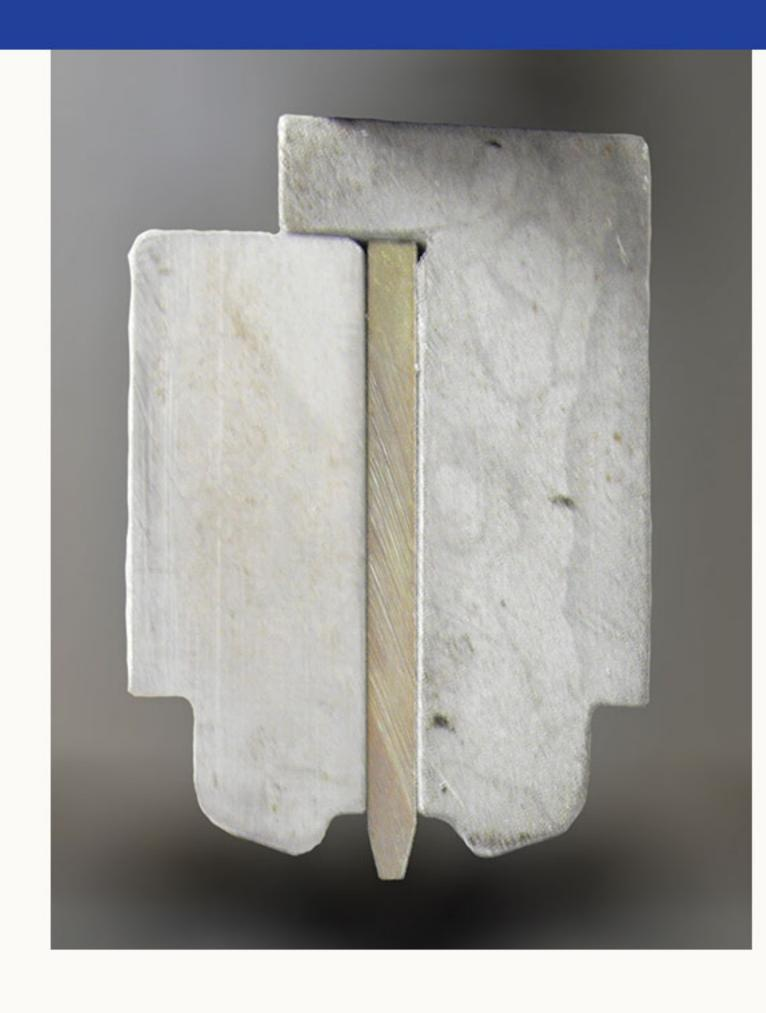
The G3 male profile features a tapered groove, which creates an area of reinforced strength adjacent to the clearly defined insert-created crease line. Because the inside liner is able to tuck into the groove, the board is forced to fold around the insert, dramatically reducing variance. Additionally, the male scorer features a three-piece design for easy replacement of the insert.
