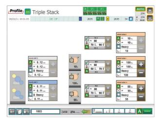
The Profile system provides accurate automatic control of produced board grades. All process parameters are monitored in real time and controlled in relation to speed or temperature via configurable graphs. Closed-loop control is achieved by analysing board profile measurement feedback.
