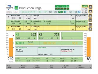
Syncro 7 can be flexibly expanded to provide the seven main corrugator supervisory objectives: wet end control, dry end control, closed-loop process control, office communications, traceability, integrated rollstock and materials handling interfaces.
